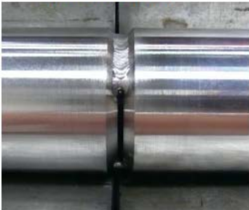
UNS N08020 Research and Weld Trials
